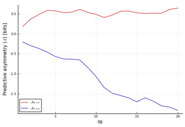
The PredictiveAsymmetry is a numerical estimation of causal connections. It works by calculating the prediction skill from one time series to the other
