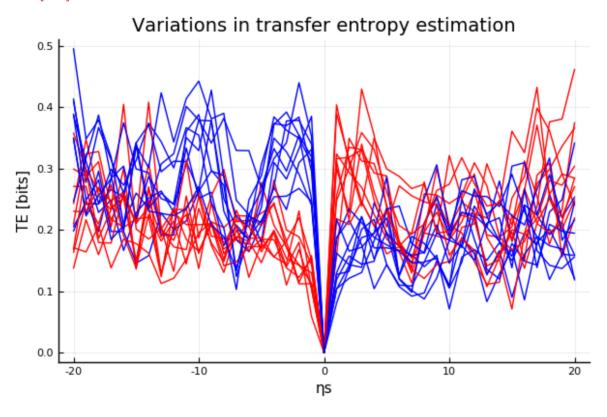
Above: **10 iterations of transfer entropy estimation.** The varition in estimation of transfer entropy stems from the stochastic component of the system, inferred by the uncertainty in the time series. Each iteration shows a series of transfer entropy values over 20 prediction lags ( $\eta s$ ) back and forth in time.
