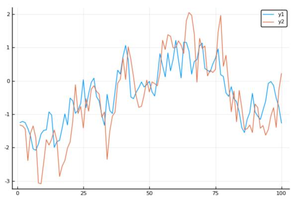
The information of the overarching dynamics defining our system's plays out in the time series of each of the system's variables. We can use delay embedding of the time series to make a state space reconstruction of the system's dynamics.
