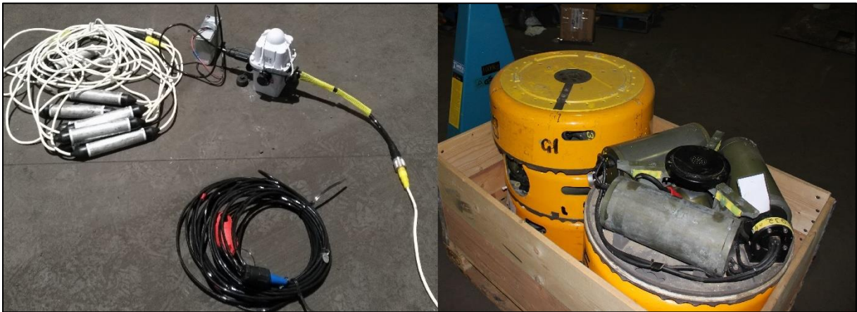
Figure 19: Some of the seismic receivers that were used during the acquisition were gimballed geophone strings (grey, upper left), Unite hydrophones (black, red and blue, lower left), and Trilobits (orange, right). In the picture to the left, a node connected to a battery is also visible.
