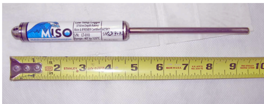
Figure 8: A low-temperature self-recording logger produced by MISO to record the temperature of diffuse, hydrothermal outflow. The temperature sensor is located in tip of the narrow rod, while the broader titanium housing contains the electronic components to keep them away from direct contact with the hydrothermal fluids. From D. J. Fornari (2009).
