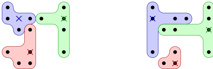
Figure 3.1: Optimal clusterings of the same set of vectors with different distances: \text{dist}_1 in the left subfigure, \text{dist}_{1/4} in the right subfigure. Shapes denote clusters, crosses denote cluster centers.
