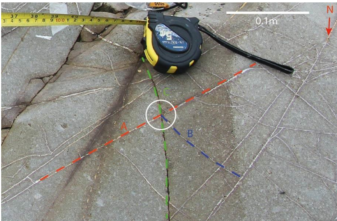
Figure 6.2: Photograph from Location 1 on the northern limb, showing an example of a situation where three fractures abut or cross-cuts at the same point, marked with a white circle. The dashed red, green
