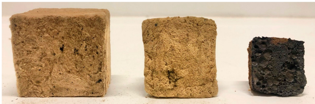
Figure 9. Test specimens after furnace heat treatments up to 1100 °C (left), 1190 °C (middle) and 1200 °C (right), as seen from the bottom of the insulation.
