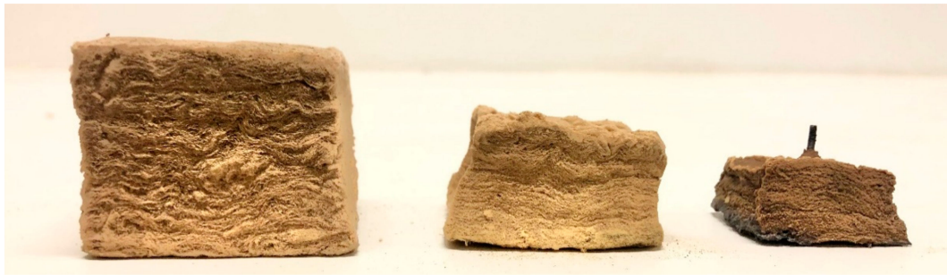
Figure 8. Test specimens after furnace heat treatments up to 1100 °C (left), 1190 °C (middle) and 1200 °C (right), as seen from the side.
