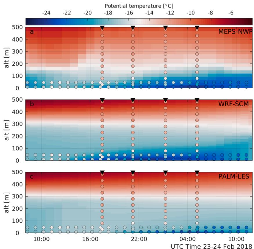
**Fig. SB1.** Time–height plots of potential temperature from the MEPS forecast (MEPS-NWP), the WRF single-column simulation (WRF-SCM), and the PALM LES simulation (PALM-LES). The data cover the lowermost 500 m and the first 24 h at the measurement site. Observations from SUMO, GFI, and FMI are superimposed as circles.
