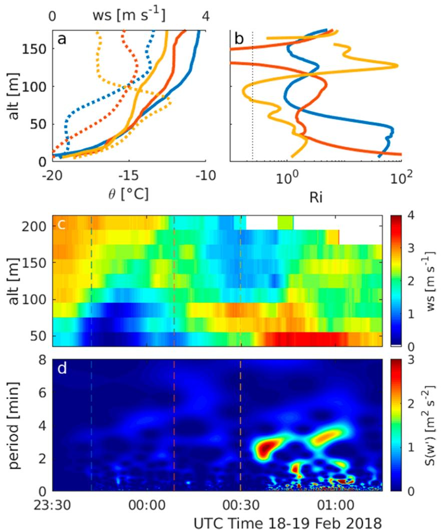
Fig. 11. Observations of (a) UAS profiles of potential temperature and corresponding lidar wind speed profiles; (b) resulting profiles of  $Ri$ ; (c) time–height diagram of lidar wind speed; and (d) wavelet energy of 10-m sonic vertical velocity component during IOP-10, 2330 UTC 18 Feb–0130 UTC 19 Feb 2018. The black dotted line in (b) indicates  $Ri = 0.25$ . The UAS flight times from (a) and (b) are indicated as vertical lines in the same color in (c) and (d).
