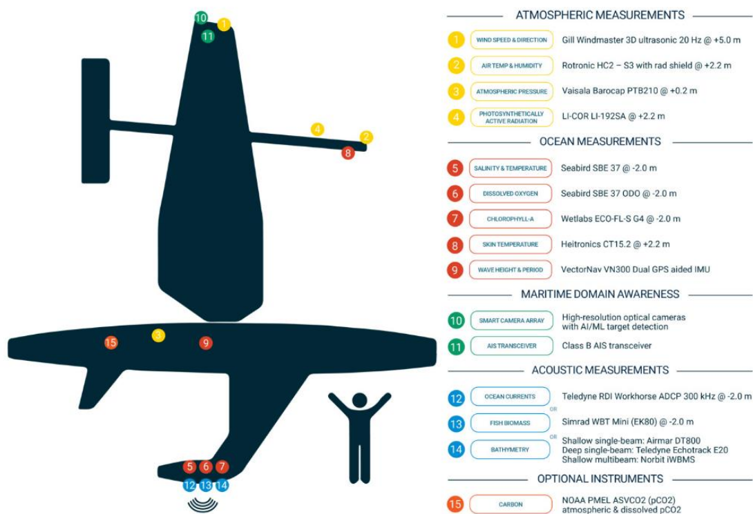
Figure 2.2. Typically equipped sensors and the installed locations (copied from Saildrone, Inc website).
