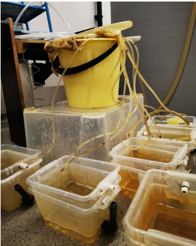
Fig. 3.2: Photo of flow-through incubator system. A 20 mm hose from the water in the level- tank was put into a sieve placed on top of the yellow bucket to filter the water. 5 mm hoses from the bucket supply filtered sea water into incubators. The inner box consisted of a bottom of mesh netting ensuring water replacement. Outlet on each incubator (black pipe on the outer box) ensure constant water replacement and determined water level in incubator.
