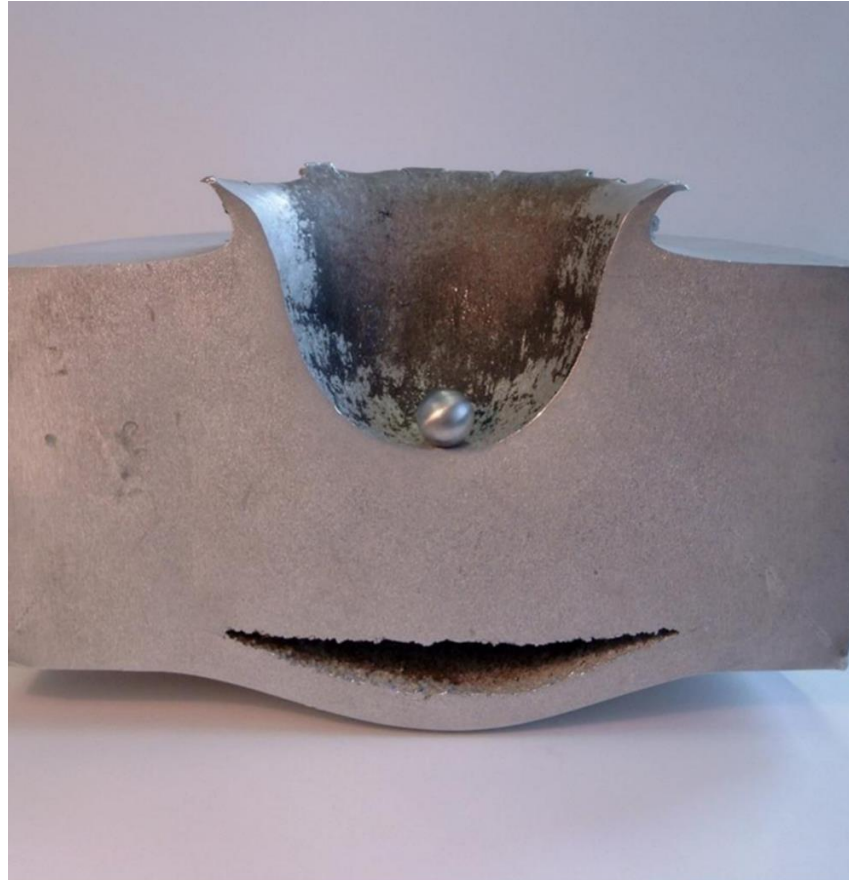
Image 1 – The impact of hypervelocity in space. The marble in the image is only 1.2 cm in diameter. The aluminium shield is 18 cm. The impact is measured at 6.8 km / s. (Credit: European Space Agency)
