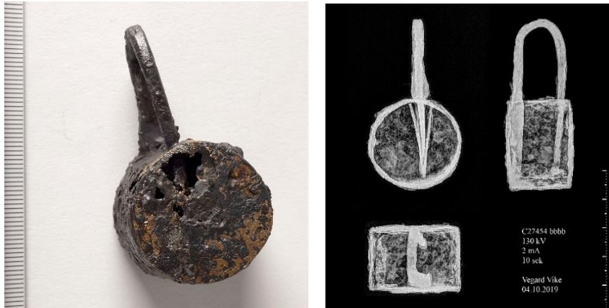
Figure 6.73. Photo and X-ray image of C4 padlock from Byggland, Kviteseid, Telemark (C27454bbbb, Photo: Kirsten Helgeland, X-ray: Vegard Vike © KHM, UiO).
