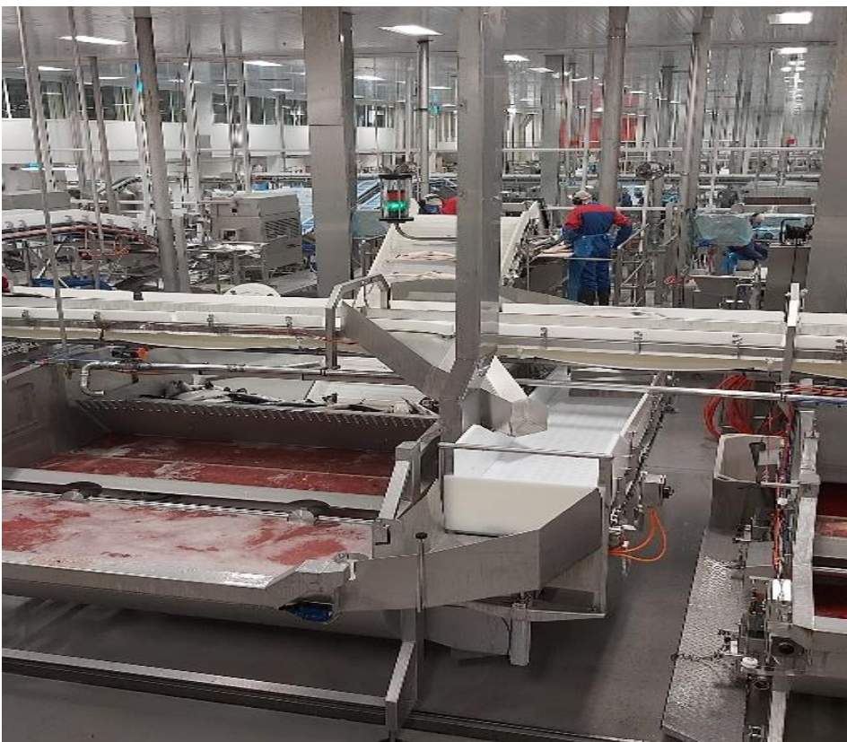
Figure 12 An example of a storage container where the fish can be storage before heading.
