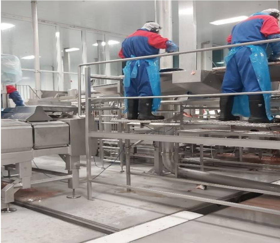
Figure 11 An example of a working station, heading machine.
