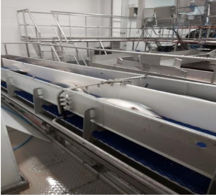
Figure 7 A part of the desliming area where the fish is rinsed after coming from the cooling tanks.
