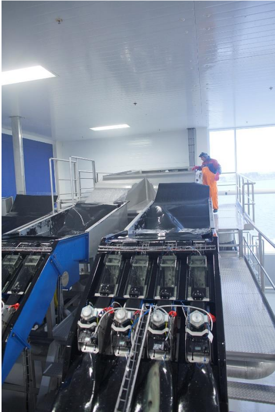
Figure 2 An example of a stunning rig. This is where the fish that is going to bleeding enters the factory and get stunned before bled.
