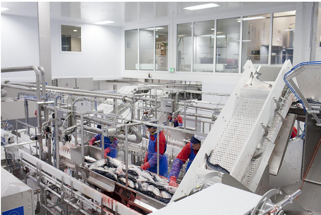
Figure 10 An example of a manual gutting working station.
