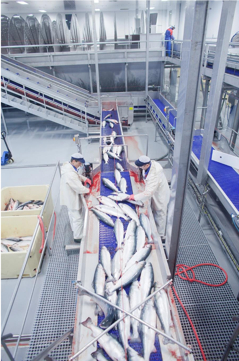
Figure 4 Overlooking a bleeding line where the fish is manually stunned and bled.
