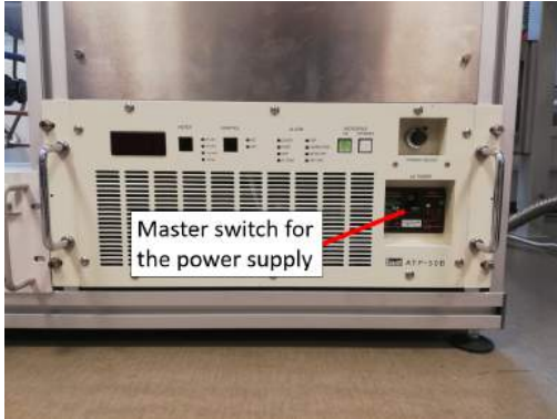
Figure 6: Shows the power supply for the magnetron.
