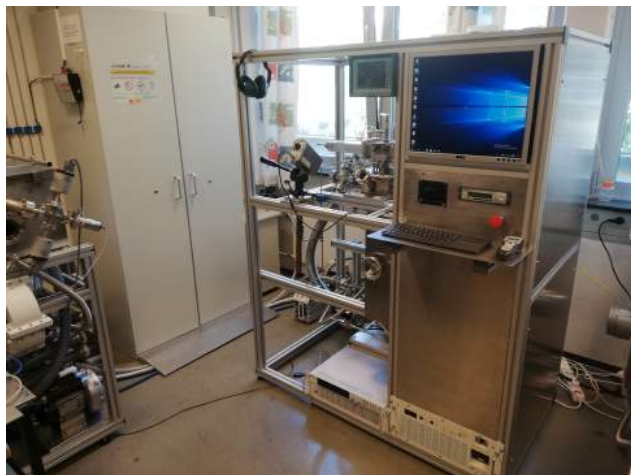
(a) The cabinet storing the hydrogen and methane is found in the left in the image. In the middle, under the window and on the floor is the vacuum pump. The deposition reactor is located in the middle of the scaffolding. And, lastly the microwave generator is found under the metal covers.
