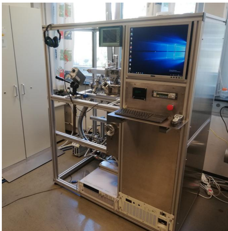
Figure 4.1: Microwave power chemical vapour deposition (MWPCVD) reactor. Further information of all the components are given in the user manual found in the appendix.
