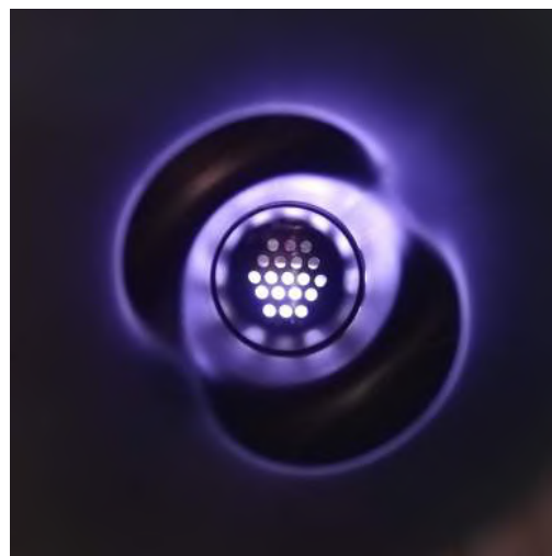
Figure 17: Shows the presence of secondary plasma seen through the secondary window of the reactor.
