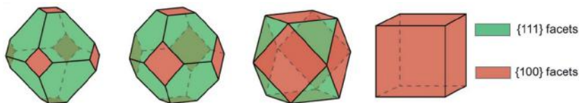
Figure 3.4: Intermediate crystal shapes between the \langle 111 \rangle shape and the \langle 100 \rangle shape [69].
