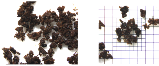
FIG. 3. Microscopic images of the investigated coffee powder. The grid cell size in the right image is 1 mm (the largest cells).
