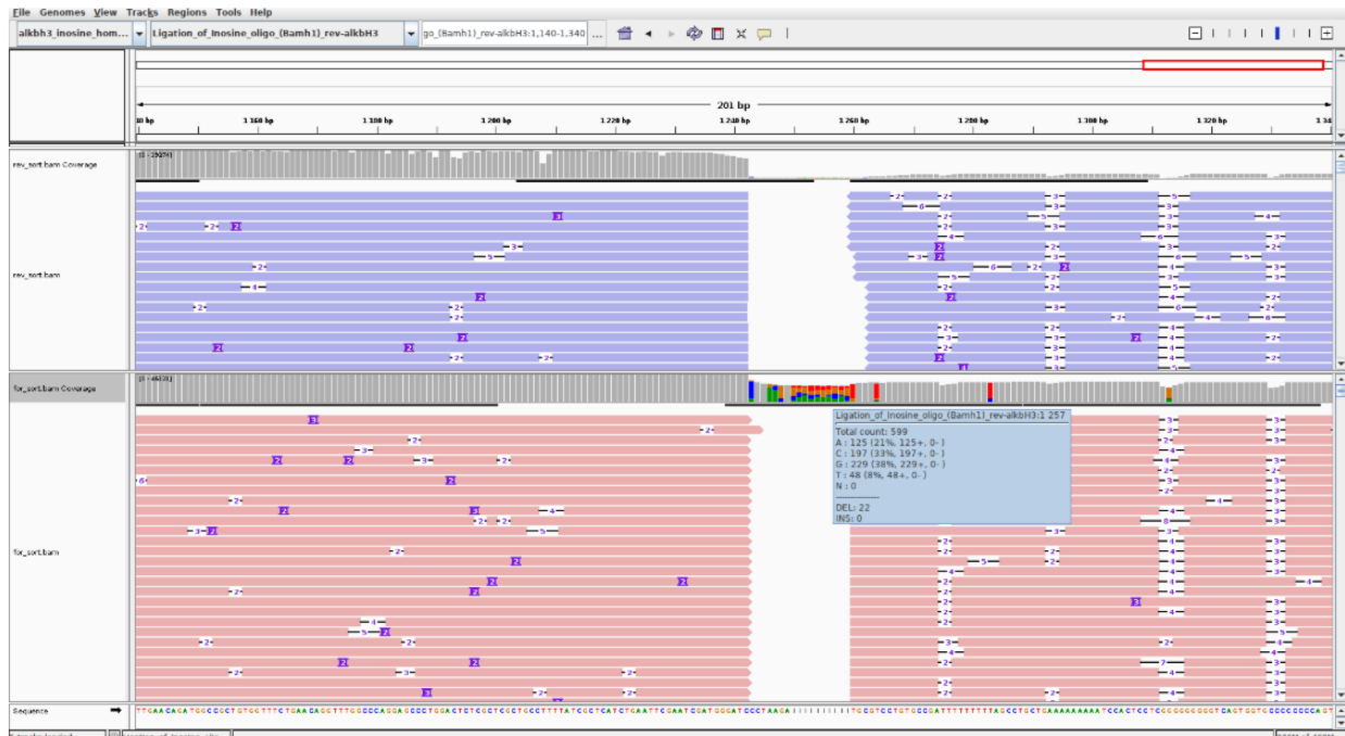
Figure 2.3: Two separate alignments viewed in IGV. The red bar toward the top shows us where in the reference we are located. Grey vertical bars on top of both tracks indicate read coverage. Hovering over these will give base counts at each position. Colored vertical bars, which can be seen above the lower construct, indicate that there is no overwhelming consensus for base identity at the given positions. The horizontal bars represent individual reads. When processing reads, aligners consider both the given reference and the reverse complement of the provided reference unless a single direction is specified. If a read aligns best with the given reference, it is labelled as a forward direction alignment. Conversely, if the read aligns to the reverse complement it is labelled as a reverse direction alignment. The direction of the read is indicated by a bit flag variable in the aligned output. In the figure above, blue horizontal bars indicate reverse alignment, and red indicate forward alignment. At the very bottom the reference sequence can be seen with small letters.
