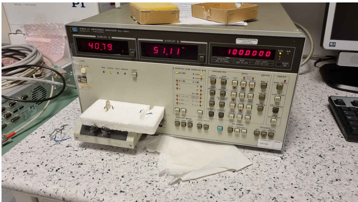
FIGURE 3.2: HP 4192A impedance analyzer used to measure the admittance of the element.
