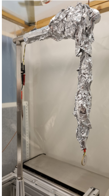
FIGURE 3.11: Transmitting element mounted in measurement setup.
