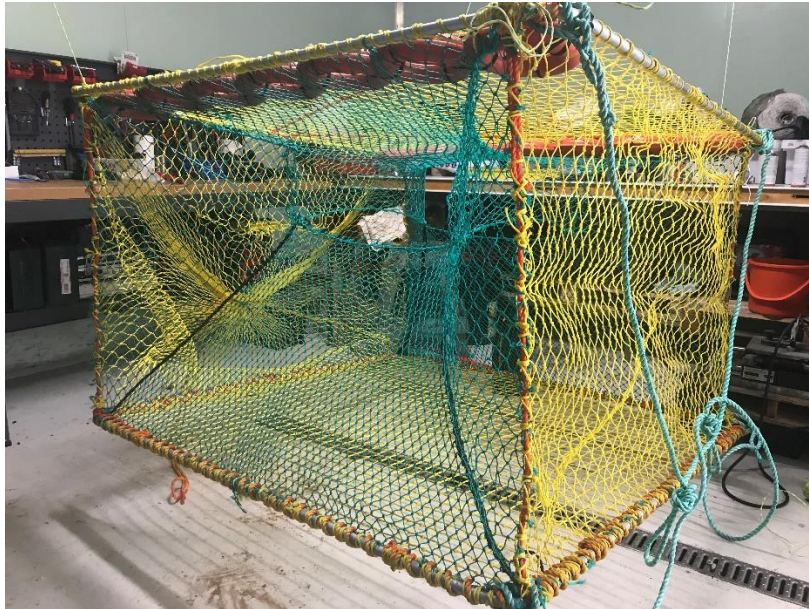
Figure 2: A Leif Henriksen pot (LH-pot), one of the standard collapsible pots used in the Norwegian Red King Crab Fishery.
