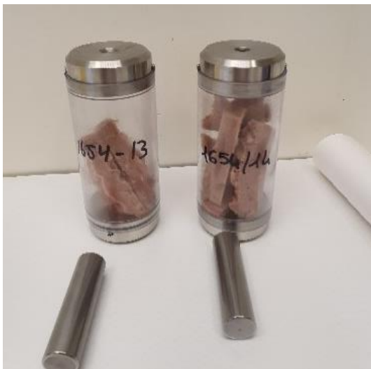
Figure 2.7.2.3 Picture of two tubes with samples inside and the rods outside, before processing with cryo-mill.
