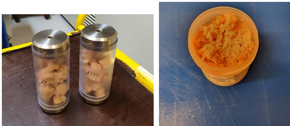
Figure 5.2.1 Frozen homogenized samples in cryo-mill-tubes before milling (left panel) and slightly thawed homogenized samples after milling (right panel).
