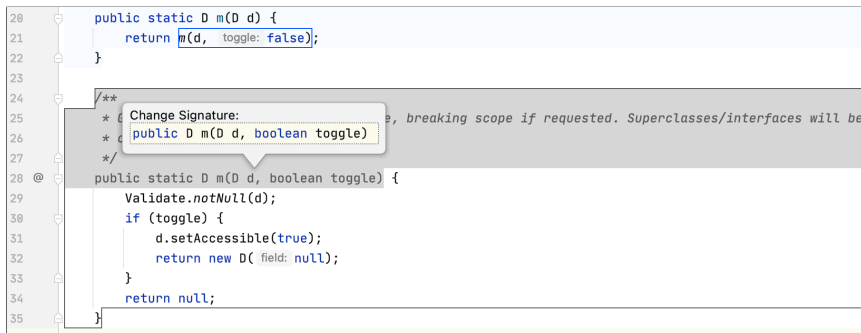
Figure 6.5: Alice invokes the stepwise refactoring tool through the refactoring menu. The tool presents an initial interface where no changes have been made. However, Alice's intent to change the method's signature has been captured and used to indicate potential impacted areas.
