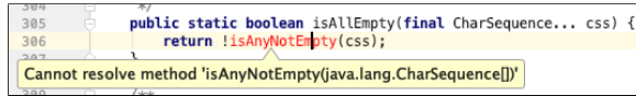
Figure 3.8: Participants who began their work on Task-2 with deleting the method and only later attempted to invoke the inline-method tool were unable to do so since the declaration no longer existed.
