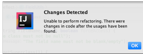
Figure 2.5: If a developer alters the source code during the preview step of a refactoring in IntelliJ, that refactoring can no longer be applied. Instead, this error is produced, and the refactoring must be re-invoked and re-configured before application.
