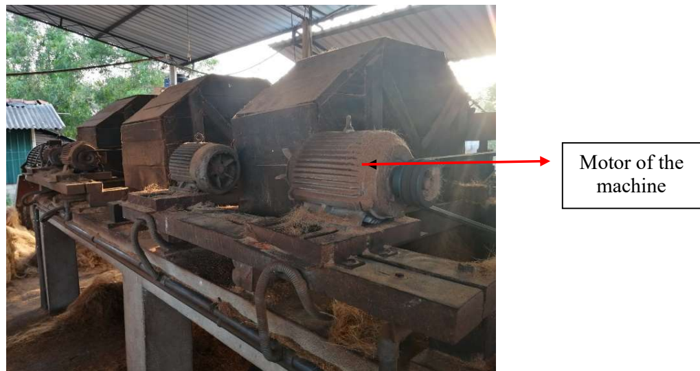
Figure 7: Traditional decorticator; It has a belt, drums, and motor using electricity.
