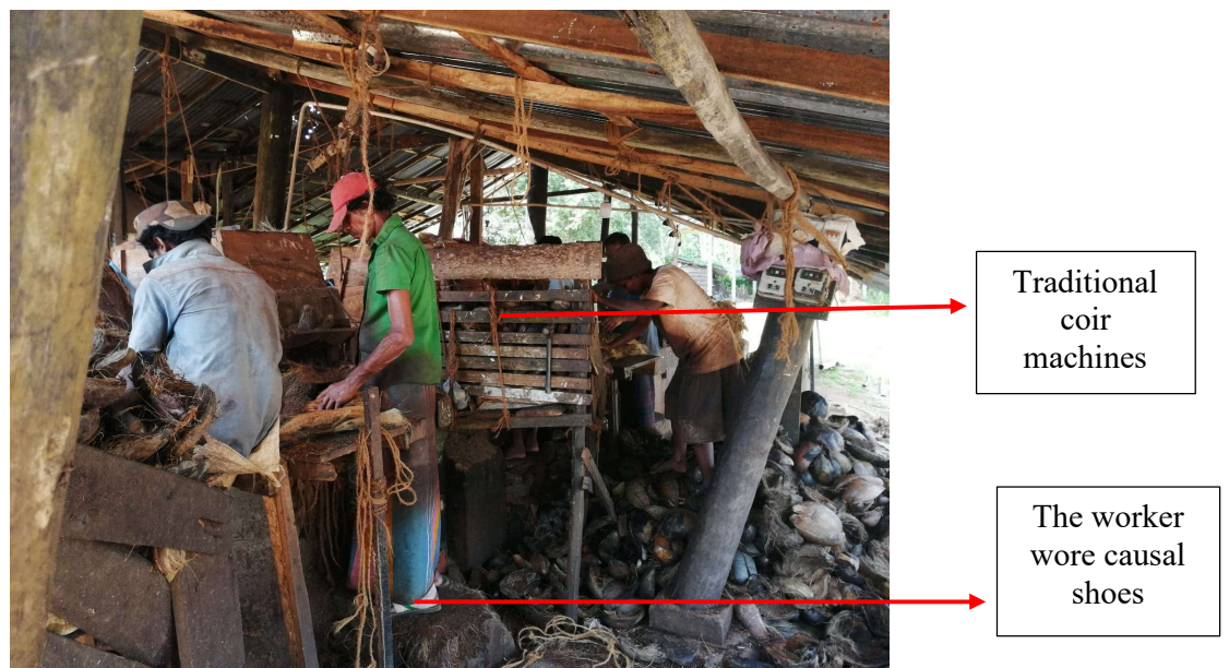
Figure 13: Inside the coir industry, where most of the workers worked with machinery without any protective clothing, hand gloves or shoes.
