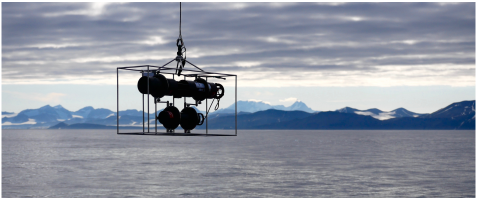
Figure 3.1: The LISST-VSF being deployed during the UAK 2020 cruise in Storfjorden, Svalbard.
