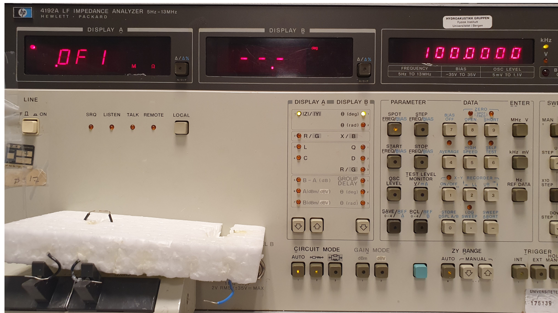
Figure 3.1: Impedance analyzer used for measurements on piezoceramic discs in air. The polystyrene foam brick is used
