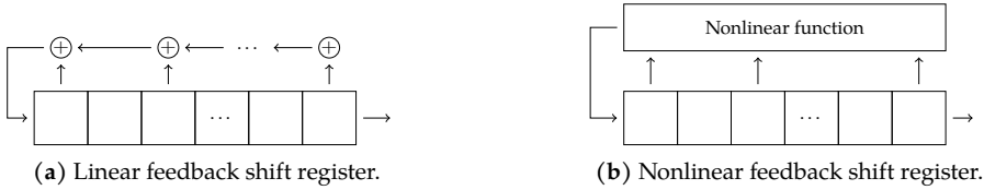
Figure 1.3. Models of feedback shift registers used in the design of stream ciphers.
