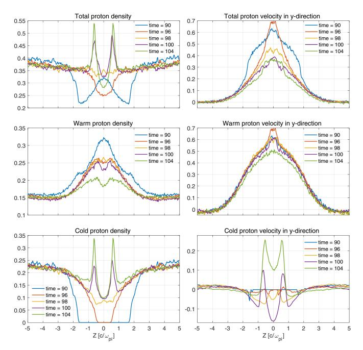
**Figure 5.** Density and *y*-directed velocity of the ion populations in the cold run as a function of *z* through the X-point at different times. The top row shows the total ion population, the middle row shows the warm ions and the bottom row shows the cold ions. The narrow peaks of positive velocity in the cold population results from the turning at the outer edge of their bounce motion.
