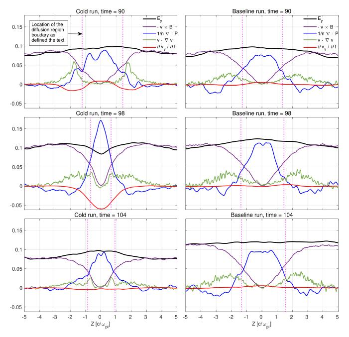
**Figure 4.** The contributing terms to the reconnection electric field as described in Equation 6 (q = m = 1), as a function of *z* through the X-point before, during and after the cold ions arrive at the reconnection site. The temporal inertia (red) has a significant contribution in the cold run, but a negligible contribution in the baseline run.
