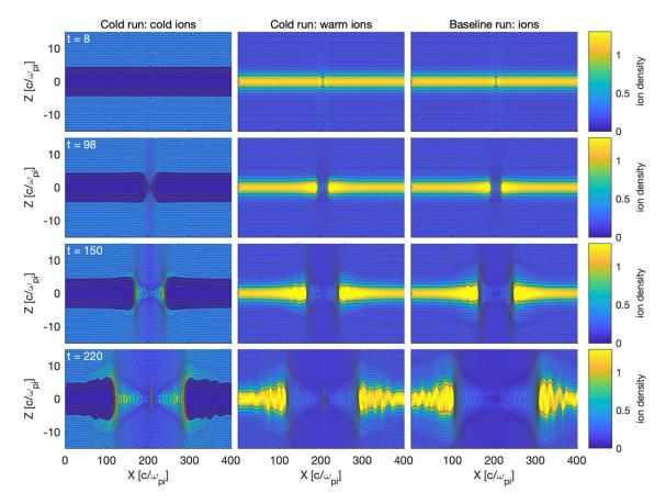
**Figure 1.** Time evolution of the ion density and the in-plane magnetic field contours in the two runs. (Left) Cold and (middle) warm ion density in the cold run. (Right) Total ion density in the baseline run. By comparing the *x*-position of the dipolarization front in the middle and right columns we see that the cold run is reconnecting slightly slower than the baseline run.
