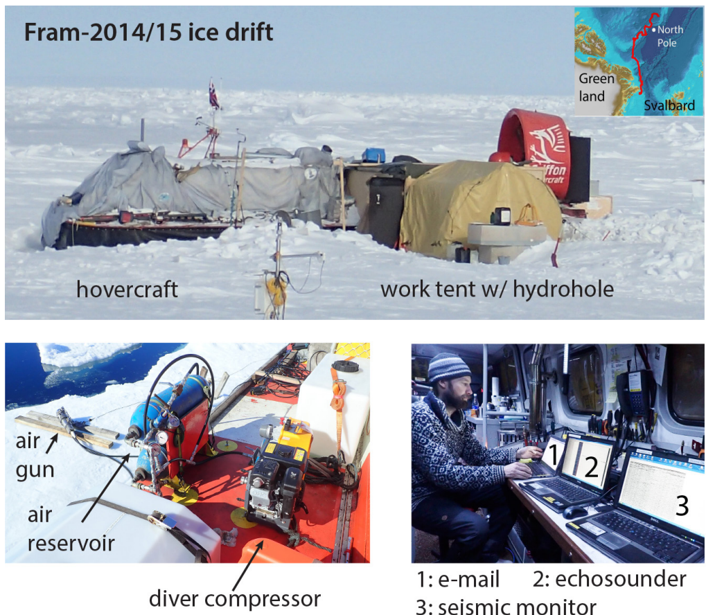
Figure 4. The Fram–2014/15 ice camp with the seismic source and data logging facilities. The hovercraft is 12 m long, has a practical hover height of 0.5 m and can carry a payload of 2.2 tons.
