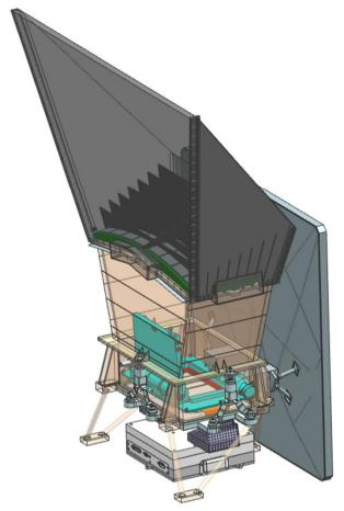
Fig. 8 CAD model of the SMILE Soft X-ray Imager and (bottom) Front End Electronics (Branduardi-Raymont et al. 2018)
