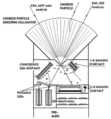
Fig. 11 IMAGE HENA instrument schematic (Mitchell et al. 2000)
