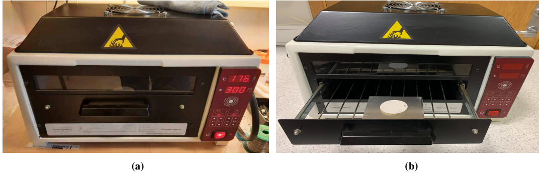
Figure 3.2: (a)The Techno HA-02 forced air convection reflow oven with the used temperature and time settings. (b) Shows how the disk is placed on a metal plate inside the oven.
