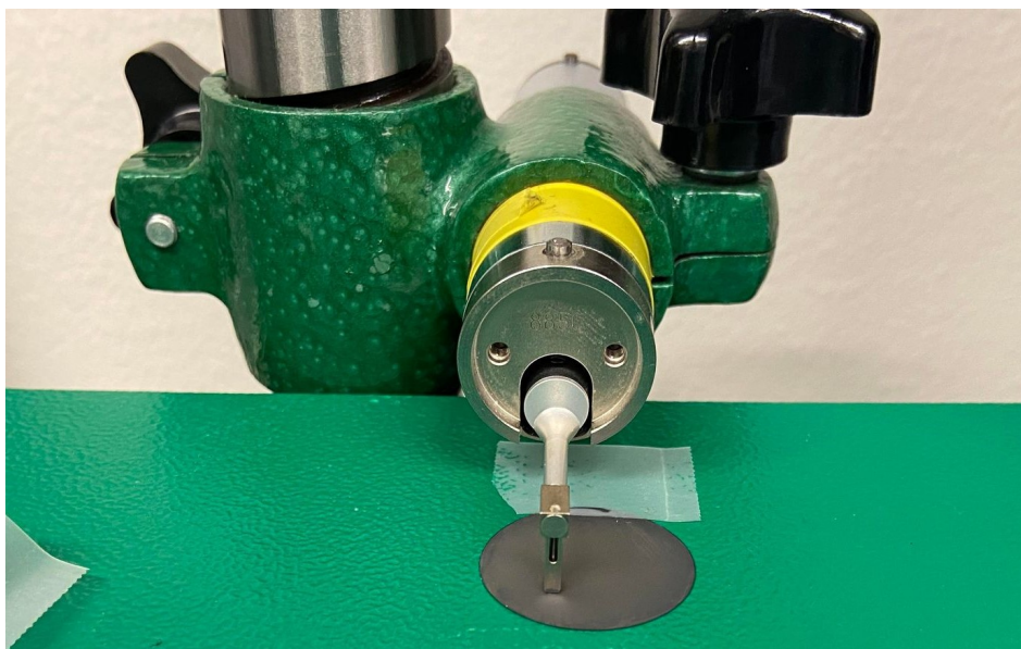
Figure 6.5: Image of the Profilometer used to measure the roughness of the microcrystalline sample S5.
