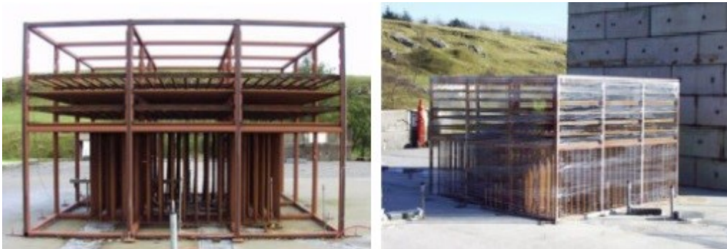
Figure 11: The congestion rig used in the experiments, congestion rig with 4-gates (left) and the rig with plastic sheet (right) [32].
