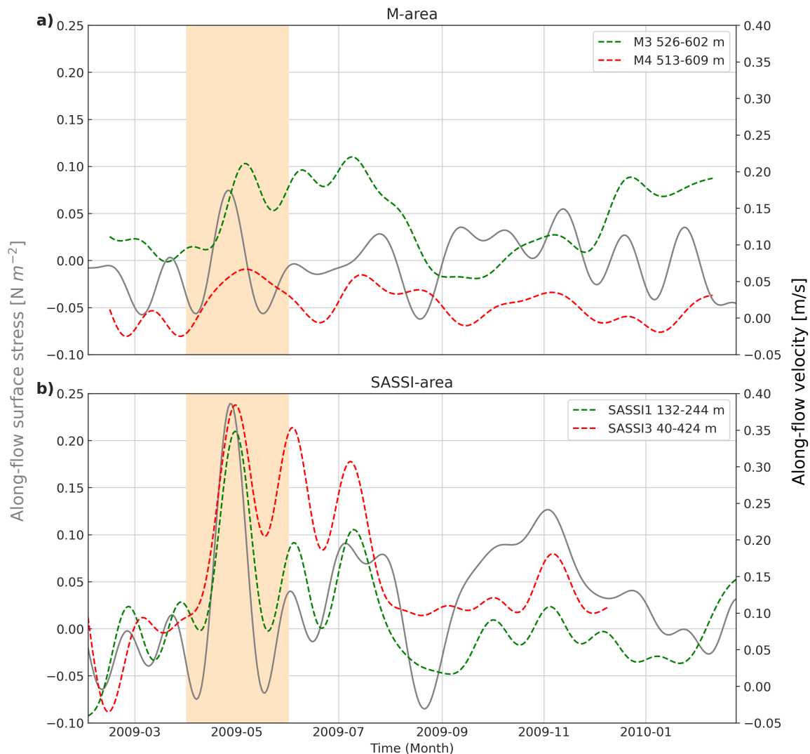
Figure 4.9: Low-pass filtered (15-days) daily surface stress along-flow(slope) in M(SASSI) area and daily along-flow velocity a) averaged in-depth ranges where we define salinity and temperature instruments in M-area and b) in SASSI-area where we use ADCP data. The rectangle (pink) is between April and June 2009, when we see the jump decrease in salinity. We calculated the components relative to the mean direction of the depth-averaged current at M3, M4, SASSI1 and SASSI2 for the whole year (section: 3.2).
