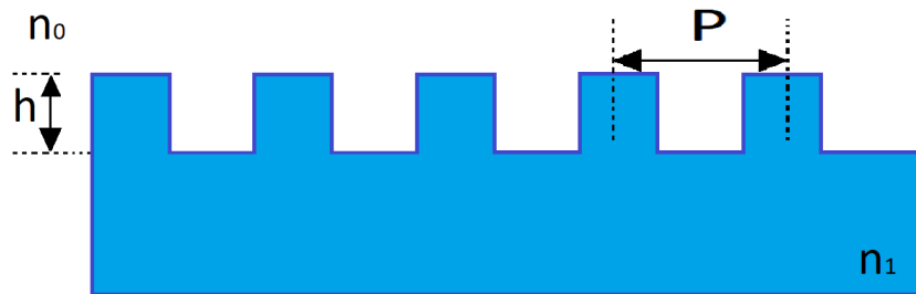
Figure 12: Sub-wavelength post illustration. Here the holes effectively halve the effective refractive index in the surface, if the posts and hole are of the same sizes. This size relationship can be changed to tailor the effective refractive index.
