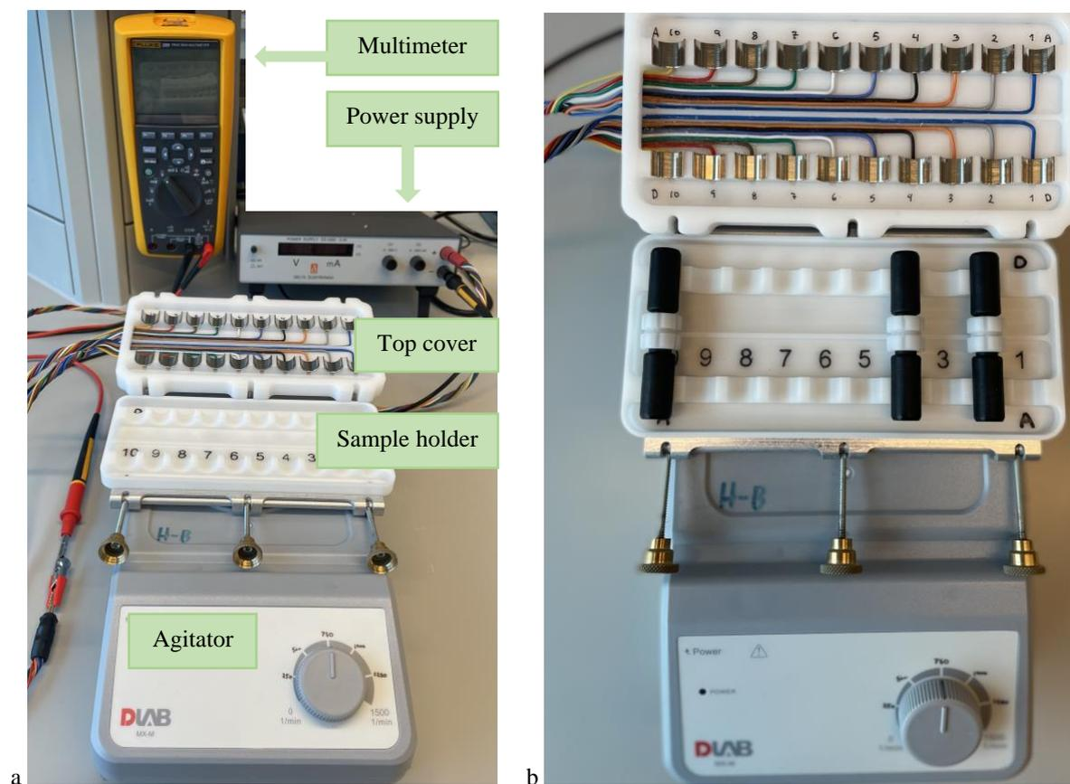
**Figure 12.** (a) EME equipment setup. (b) Top cover with electrodes and sample holder with 3 samples.
