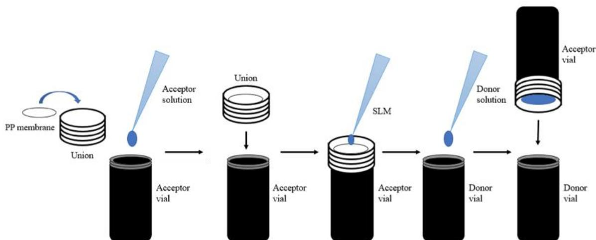
**Figure 13.** Schematic view of the EME procedure. Adapted and modified from (46).
