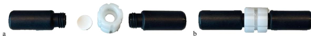
**Figure 11.** (a) Sample equipment prior to assembly, from the left: acceptor vial, flat sheet PP membrane, union and acceptor vial. (b) The assembly of a sample unit.
