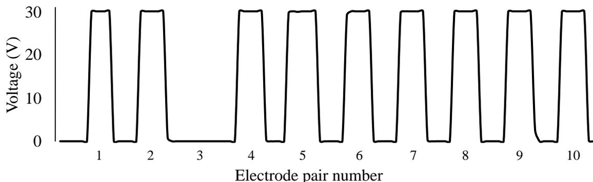
**Figure 19.** Measured voltage (V) of the electrode pairs at 30 V.
