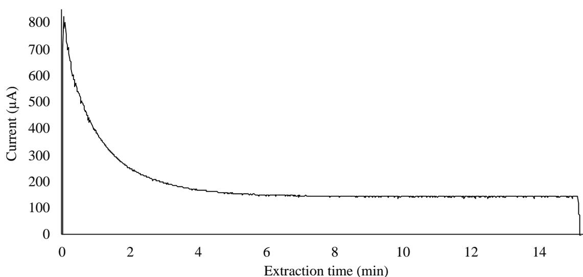
**Figure 14.** Example of a stable EME current curve with nine samples extracted simultaneously at 30 V with a variation of extraction conditions. This is taken from an experiment performed at the University of Oslo.
