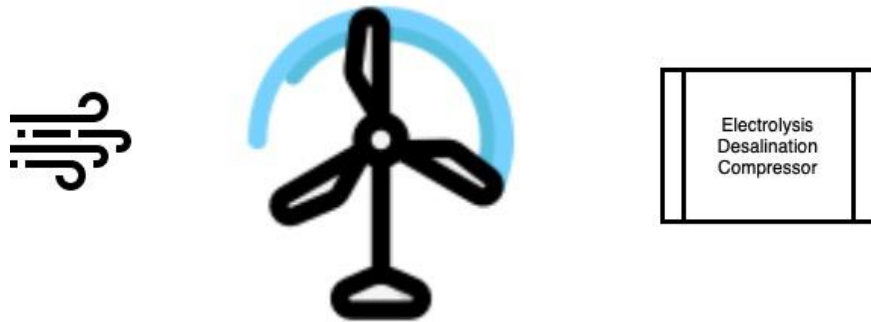
Figure 16: Case 2: System overview; large-scale hydrogen production system
