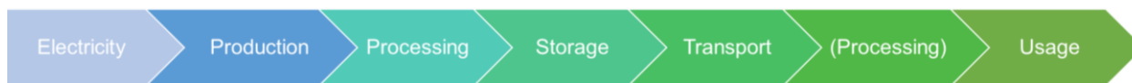
Figure 1-1 - Hydrogen value chain for production through electrolysis. This illustration shows the many steps related to the hydrogen value chain, which include production, processing, storage, transport, possibly re-processing and then either use directly in industrial processes or combustion, or in a fuel cell to produce electricity. Processing is indicated with a parenthesis after transport, as only some hydrogen carriers require re-processing.
