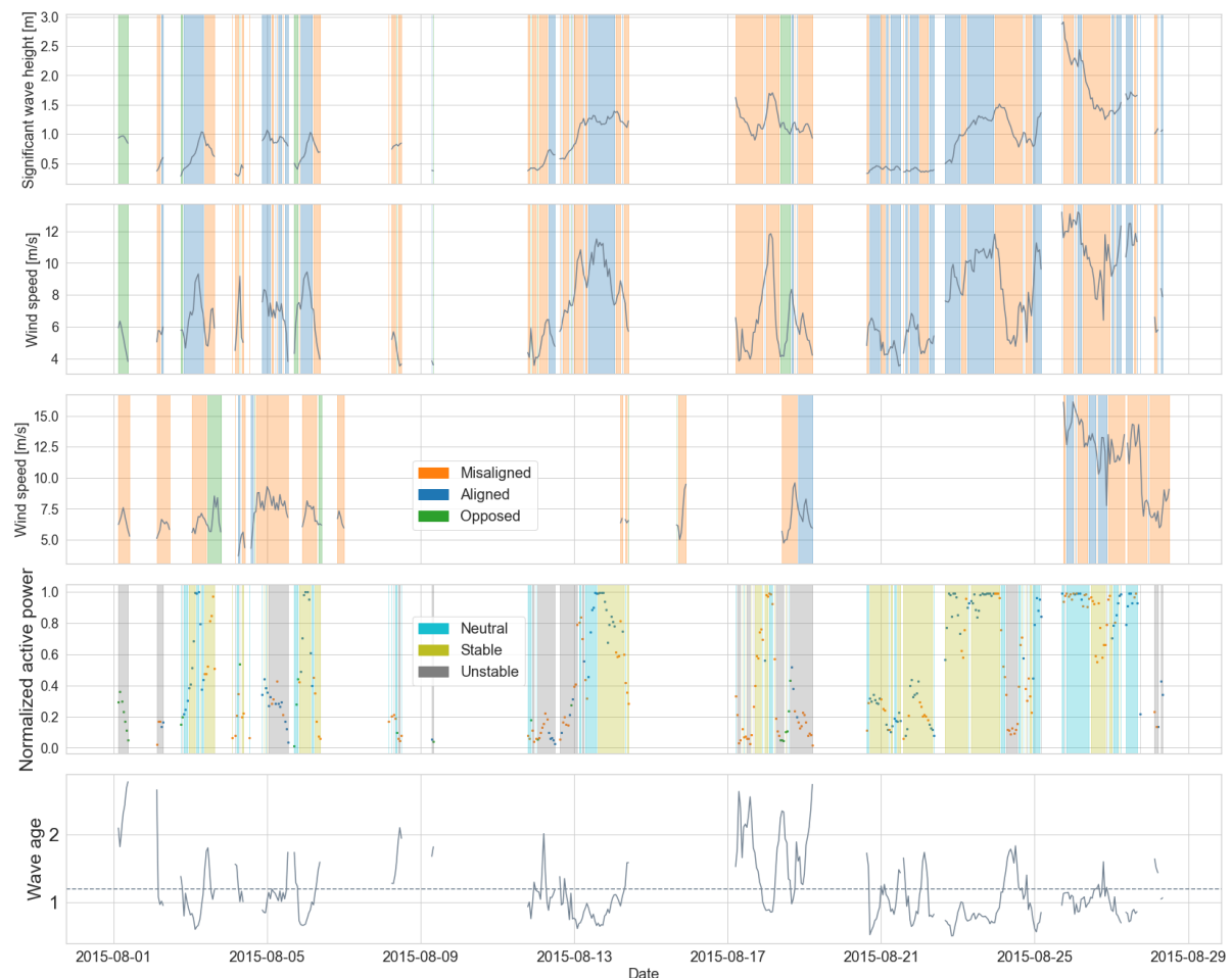
Figure 5.14: Wind-wave alignment and stability: For the upper three plots, wind-wave alignments are shown. The top plot shows significant wave height, followed by wind speed at 15 m and 80 m. The last two plot shows atmospheric stability at the height of 80 m and wave age.
