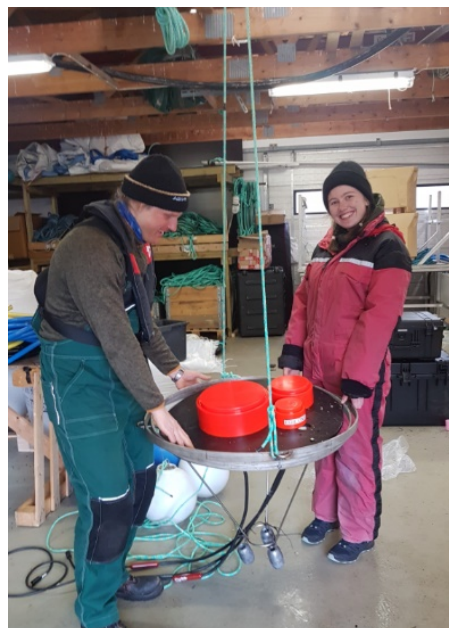
Figure 3.3: Transducer setup and gimbal, illustrating how the transducers were facing upwards when placed underneath the cage
