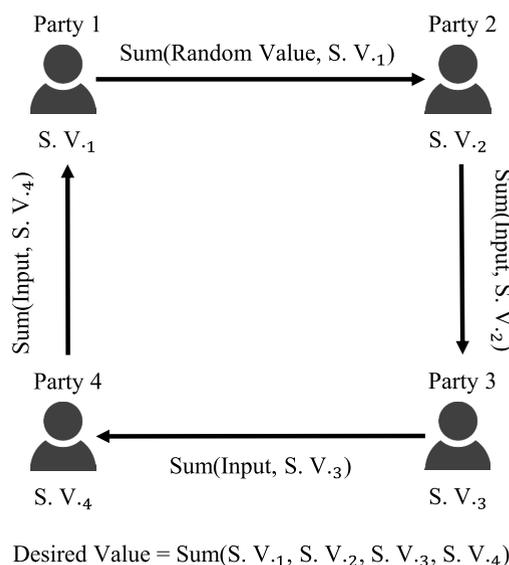
**FIGURE 1. Secure aggregation.**
