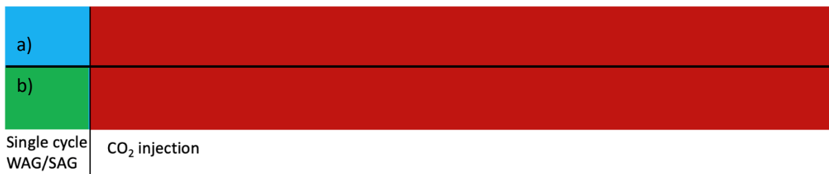
Figure 7.3 Single-cycle WAG and SAG injection where a) represents the WAG injection with brine and b) represents the SAG injection. The total injected volume is equivalent to 10 pore volumes.
