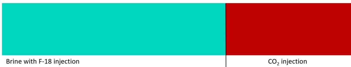
Figure 7.5 Schematic of the baseline injection of 2PV of brine, followed by 1 PV of CO 2 .
