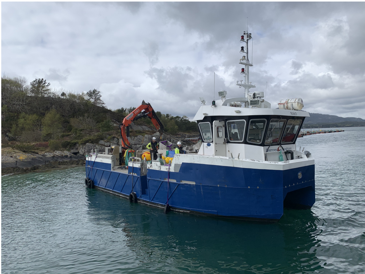
Figure 5.10: The workboat Randi used to deploy and recover the mooring is 14.99 m long with a crane and winch installed on deck.
