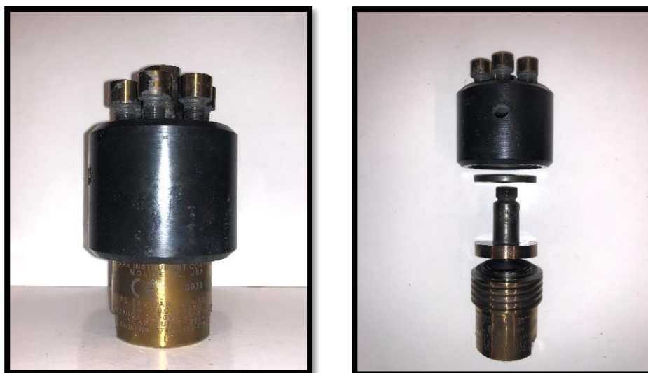
Figure 3.3-a: Picture of the 25 mL volume batch reactor, both assembled (L) and dismantled (R).
