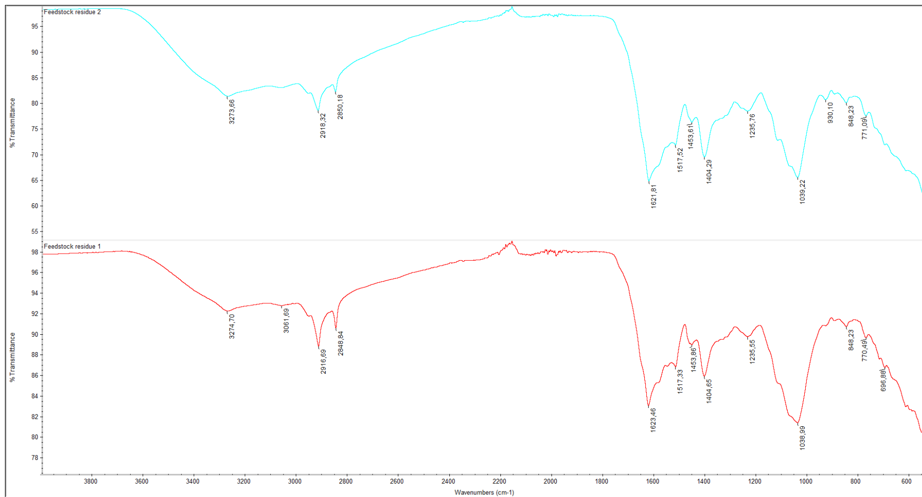
Figure C.5-a: Comparison of the IR spectra for Feedstock residue 1 and 2 from Soxhlet extraction.
