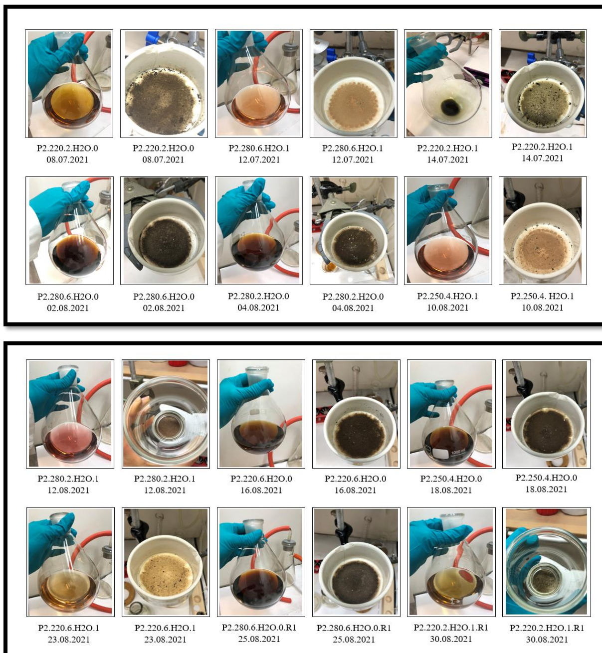
Figure 4.3-a: Pictures of the oil (diluted in solvent) and coke samples from the experimental work-up from P2.
