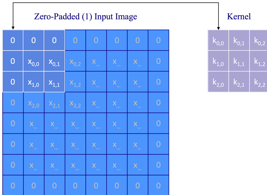
FIGURE 3.20: A Zero-Padded input image with only one pad. The zeros that create a border around the image allow the kernel to center on the edges of the original input array.
