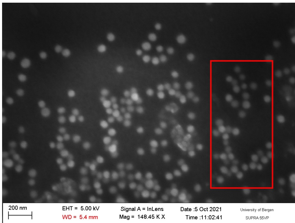
Figure 4-13: SEM analysis of 60 nm gold nanoparticles from NanoComposix (Zeiss Supra 55 VP). In red rectangle: Particles measured with ImageJ.
