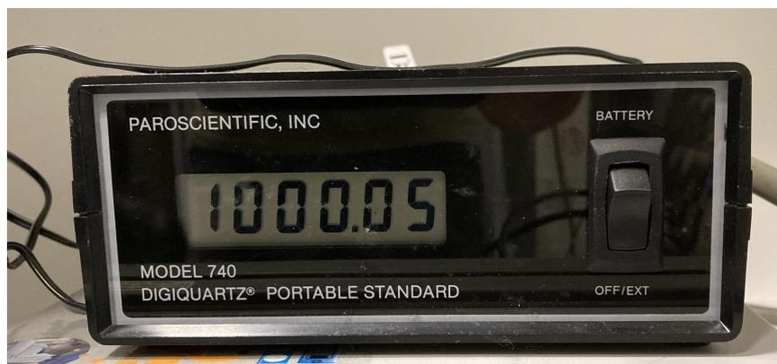
Figure 3.35: Picture of the Paroscientific Digiquartz precision pressure instrument model 740 used for pressure measurements.
