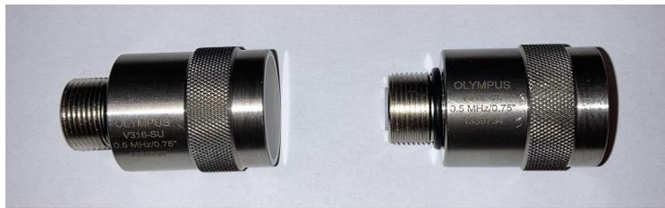
Figure 3.3: Picture of the two V318-SU transducers used in this work.
