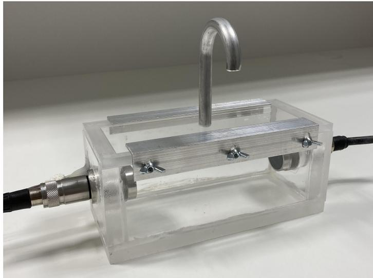
Figure 3.14: The final design of the measurement cell.
