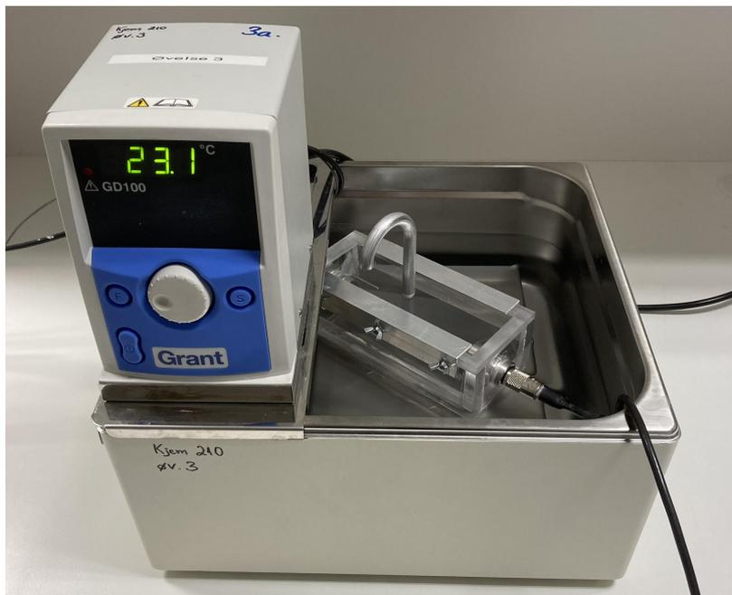
Figure 3.9: Picture of the Grant Instruments' GD100 general stirred thermostatic waterbath.
