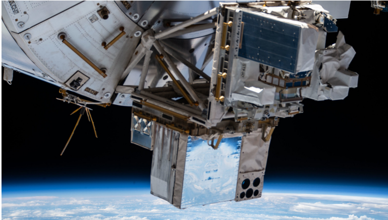
Figure 4.6: Picture of the ASIM instrument, after it was moved in 2022. The previous location was on the platform to the right, pointing downwards. The MXGS is behind the reflective square, and the MMIA is seen on the right, consisting of the 3 photometers (three circles towards the bottom of the picture) and 2 cameras (two circles above the other three). Image from https://asim.dk/images.php , visited 20.05.2022
