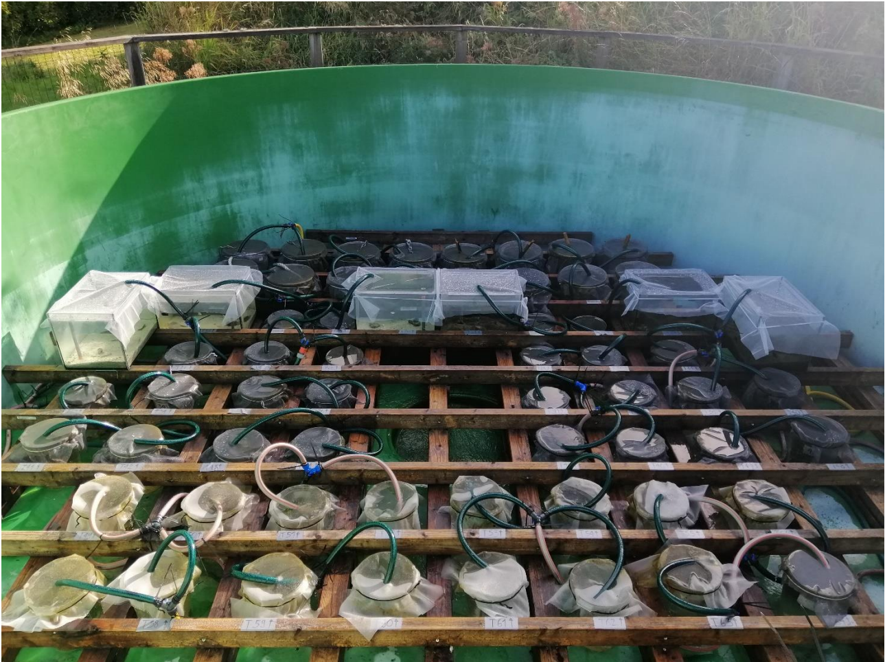
Figure 1: Experimental set-up at the Marine Biological Station Espeland. Constant sea water supply from 10 m depth provided the 64 beakers and aquaria with nutrients and oxygen.
