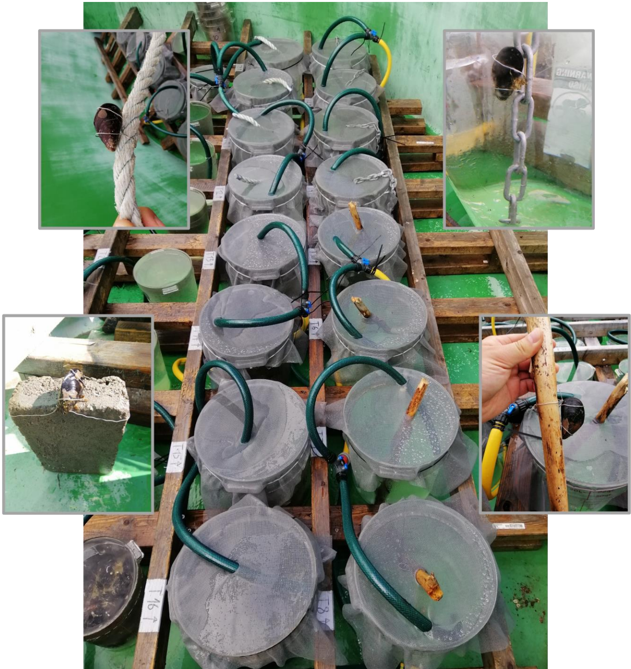
Figure 10: The set-up of the walkway experiment with four simultaneous replicates of each treatment: rope, chain, concrete brick, and branch.
