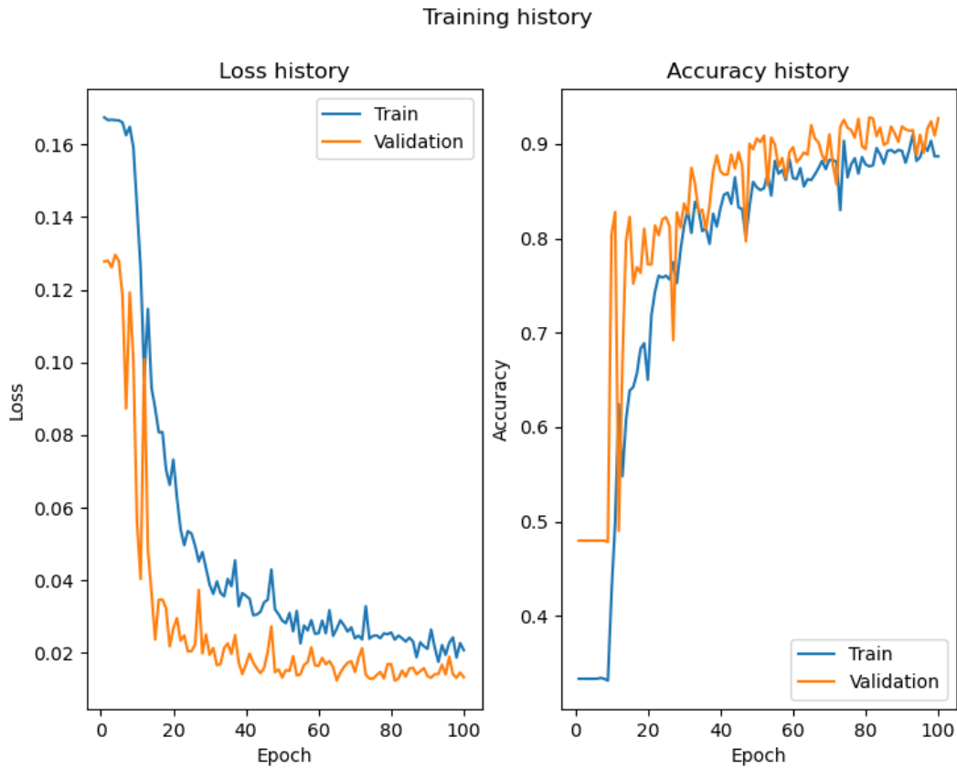
Figure 4.9: Loss and accuracy curves for the regression task using the face crops.
