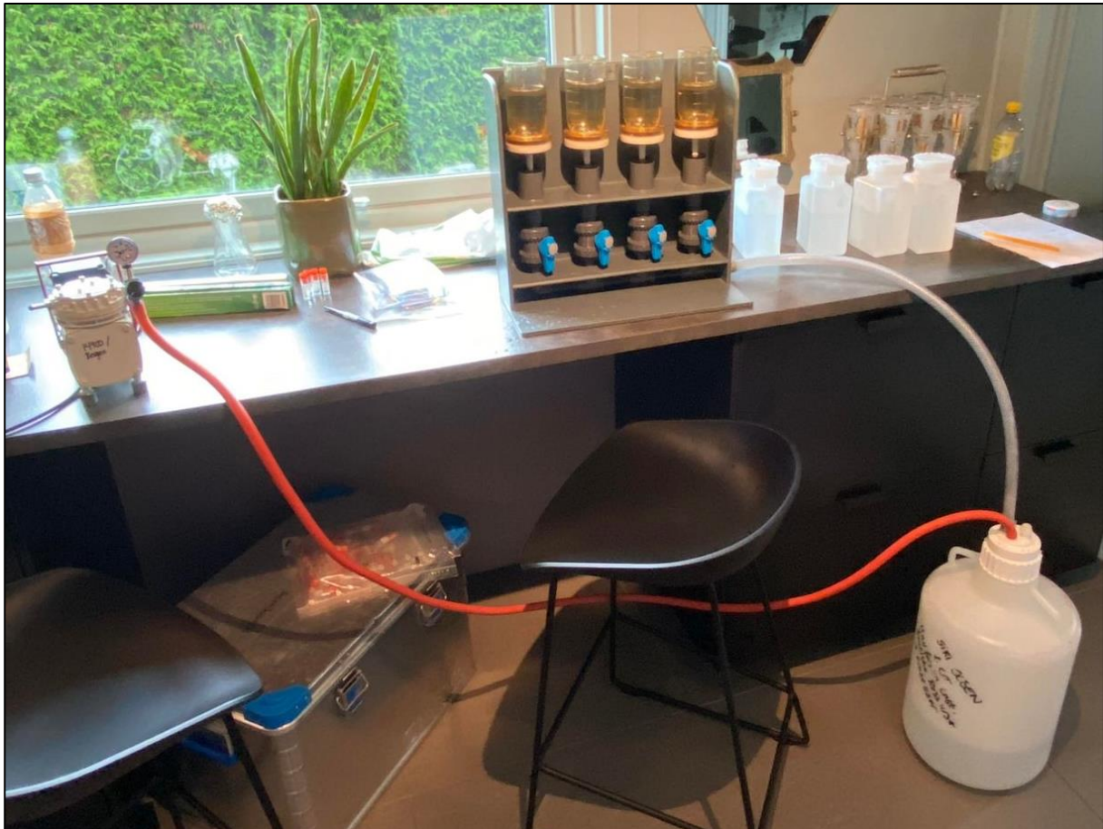
Figure 2.2: Filtration set-up during field campaign September 2021. From the left: a vacuum pump was connected to the collection tank via the outgoing orange hose. The ingoing white hose was connected to the filter stands. The four white containers to the right for the filter stand were used to transfer water from “field buckets” to the 3 dl cups.
