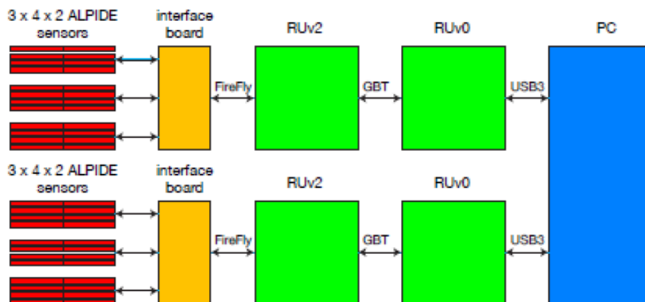
Figure 4.4: Schematic view of the readout system of the EPICAL-2 detector. [29]
