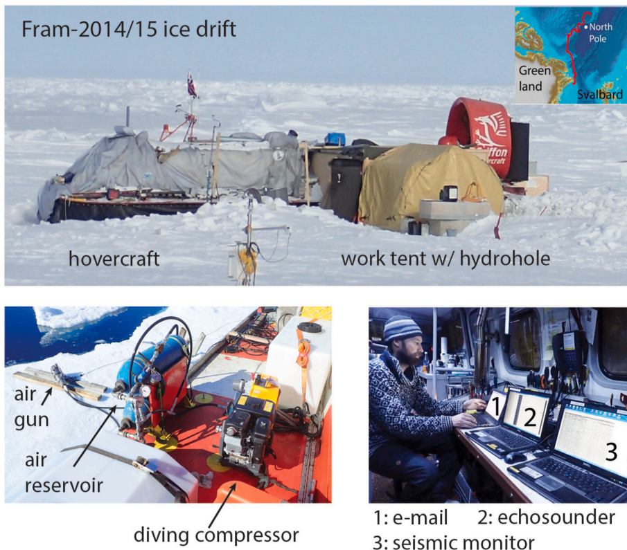
Fig. 3. The hovercraft ice camp (upper) with the seismic source (lower left) and the recording instruments (lower right).
