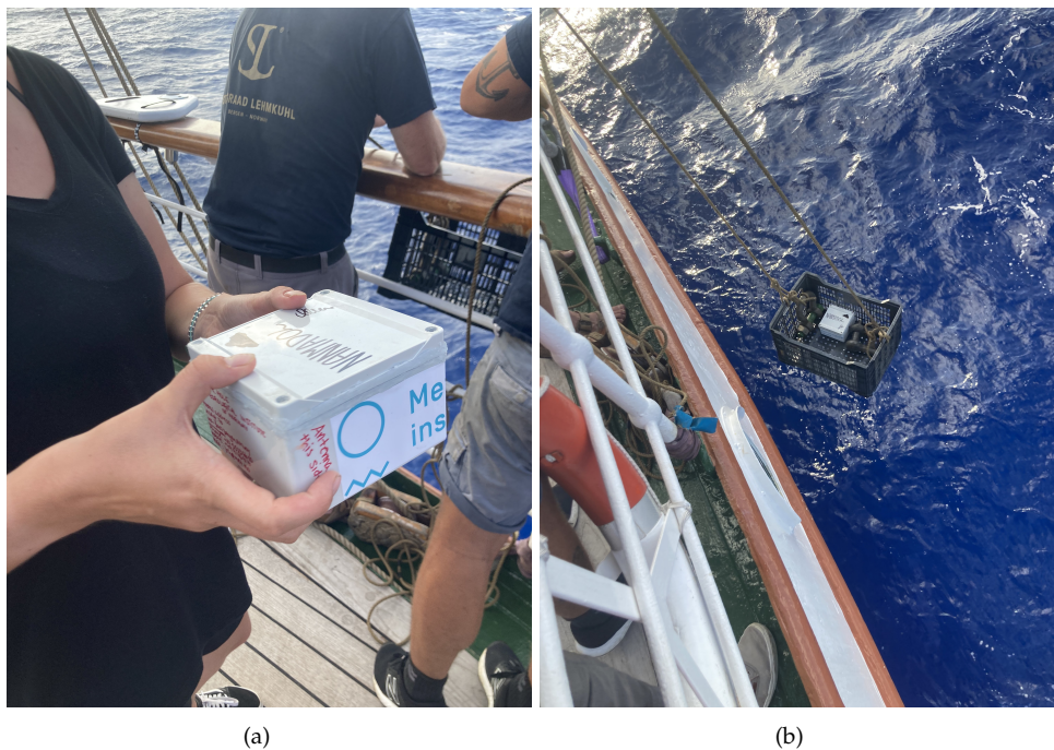
Figure 7: Picture of (a) the drifter and (b) the deployment method in a box attached with ropes.
